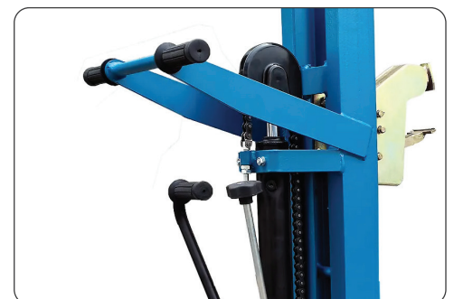
Ergonomic grip handle and height control knob
