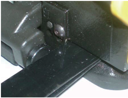
INSERT THE STRAP INTO THE SEALING SECTION AGAINST THE FRONT STRAP STOP.
