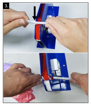
Twist plastic bag and push twisted bag down through the neck. The blade will cut the tape automatically.
