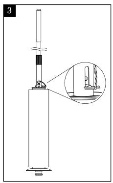
Push the film roll firmly against the top cap. Secure the film roll by inserting the lock pin in the proper hole.
