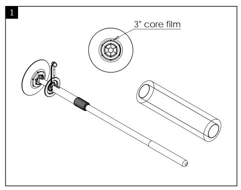
Pull the lock pin out before installing the film roll.
