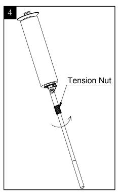
Turn the tension nut clockwise if you want to increase the tension to the film. Turn the tension nut anticlockwise if you want to decrease the tension to the film.
