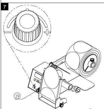
Label feeding speed can be adjusted by turning (19) speed control knob. Turn clocwise to increase speed. Turn counter-clockwise to decrease speed.
