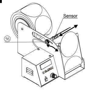
Sensor can be moved backward or forward by adjusting at side. Sensor can also be moved to the left or to the right by hand. Adjust the sensor according to the width and length of label to achieve smooth operation as labels are removed.
