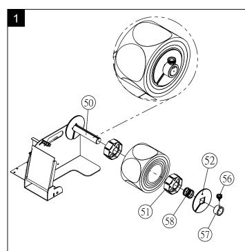
Install 51 core holders in each side of label roll.Put the label roll to the 50 spool rod.Secure the label roll with 58 spring 52 shield, and 57 collar.Tighten collar with 56 knob.
