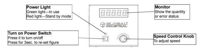
Turn on the on/off button at back of dispenser after install the label sticker. The monitor and power light turn red meaning the dispenser is ready to be used. Set up the speed and press the power switch at front, the power light turns green meaning the dispenser is in use.
