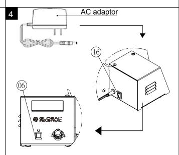
Plug in the AC adaptor to the tool and wall socket. Turn the power on (6) on/off button in the back of tool) first and then press 6 power switch in front of tool. The light on top of power switch turns green.
