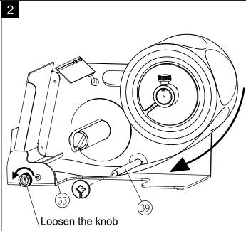
Loosen the knob in front of tool so it is easier to feed label under 39 guiding bar then between the 33 compression plate and main plate as shown.
