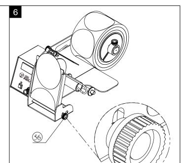
To apply proper amount of tension for proper label feeding and detection, raise 56 knob up to increase tension, then tighten the knob.
