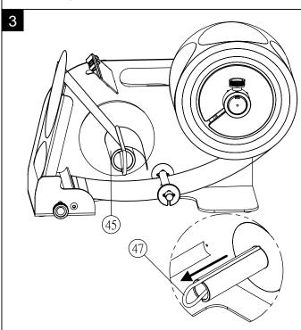
Remove (47) spring cilp.Feed label over metal plate in front of the tool.Separating the liner from the label.Coin the liner to (45) take-up hub roller.Slide (47) spring clip back on over the liner.
