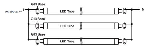
• **Fourth Step:** Affix the field applied label to the light fixture. Then install the tube. The tube is double port wiring connection
