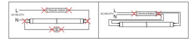
• Third Step: Install the LED tube and make the electrical connection
