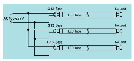
• **Fourth Step:** Affix the field applied label to the light fixture. Then install the tube. The tube is single port wiring connection.
