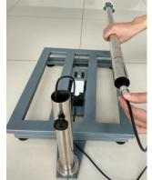
6. Insert the longer post into the short post till reach or pass the black line marked on longer post, then secure it by locking the knob.
