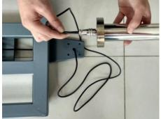
4. Secure the post onto the bracket of scale base with the 4 inner hexangular set screws. Make sure the screws are securely tightened.
