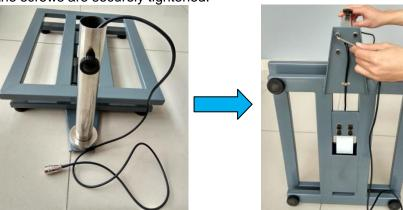
5. Loosen the locker knob on the shorter post, then insert the cable through the longer post.
