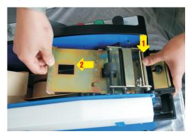
**Step 5** Press the cutter lightly and insert the tape, positioned gummed side down, through the paper feed roller. *See tape threading diagram*
