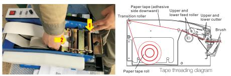
Step 6 Press the cutter lightly and install the top board back.
