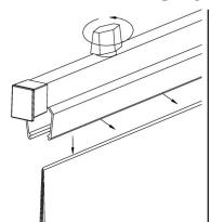
2. Insert files into clamp jaw and hand tighten wing knobs until the files are secure. Print clamp shown is a cut-away diagram to show the internal mechanism.
