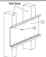
1. Locate wall studs and attach rack (part 1) using six (part 4) screws. If you cannot locate wall studs we suggest you attach the rack to a solid wall surface. If you cannot locate the studs or are unable to attach to a solid wall surface, we suggest that you have the rack installed by a professional using hollow wall anchors.
