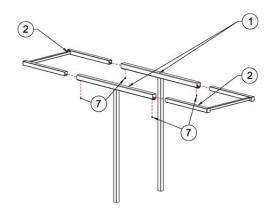
**4.** Slide upper frames into lower frames. Adjust to size of clamp being used and fasten two knob screws (part 7) into lower tube assembly.
