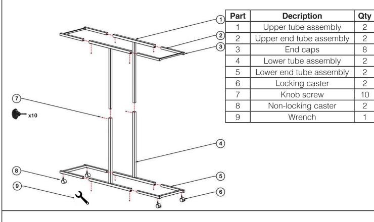
**1.** Insert lower end tube assemblies (part 5) with caster weld nuts facing down into lower tube assemblies (part 4). Adjust to size of clamp being used and fasten four knob screw (part 7) into lower tube assembly.
