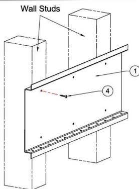
1. Locate wall studs and attach rack (part 1) using six (part 4) screws. If you cannot locate wall studs we suggest you attach the rack to a solid wall surface. If you cannot locate the studs or are unable to attach to a solid wall surface, we suggest that you have the rack installed by a professional using hollow wall anchors.
