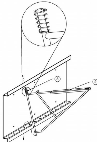
2. Guide hangers (part 2) with springs (part 3) into the top of the upper frame assembly as shown in diagram. Push upper end with spring into upper hole and then insert lower part of hanger into bottom hole of rack.
