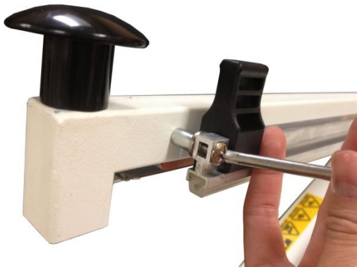
Figure 8. Unscrew the silicone bracket and remove screw, washer and spacers.
