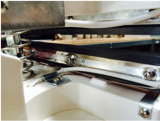
Figure 6. Loosen screws found on sealing jaw.
