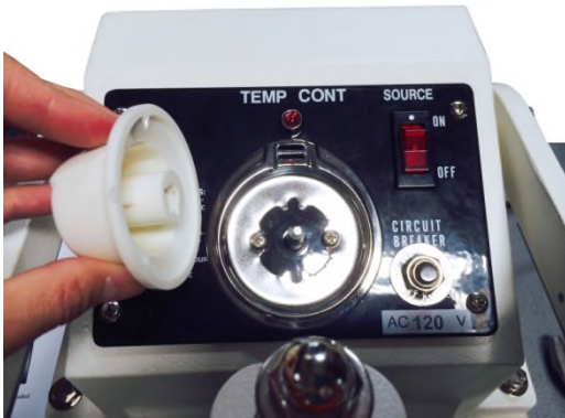
Figure 8. Remove thermostat cap.
