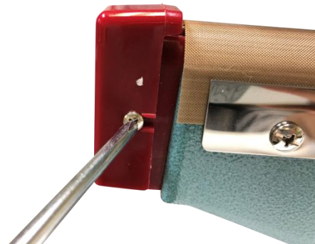
Figure 8. Remove heating element cover
