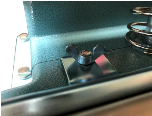
Figure 10. Loosen knob to remove the PTFE roller.
