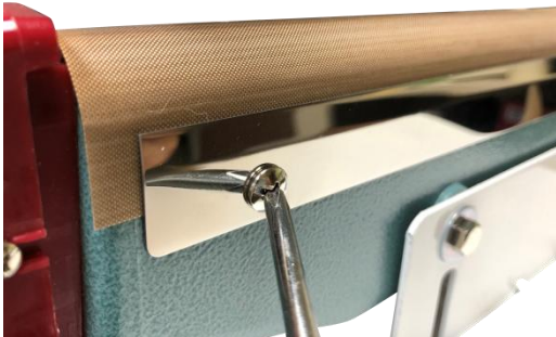
Figure 7. Loosen screws on PTFE plate.
