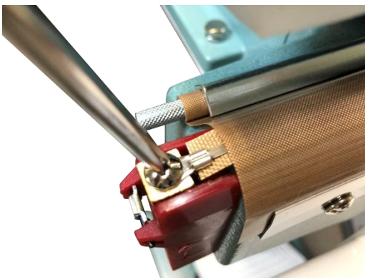
Figure 9. Remove heating element from terminal assembly
