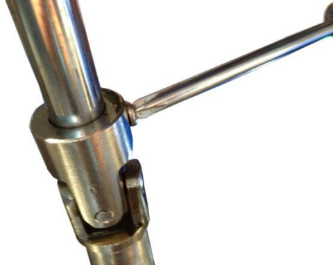
Figure 7. Screw the long shaft to the umbrella gear base.
