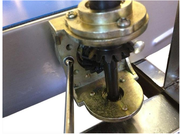
Figure 32. Set the three screws back on the umbrella gear.
