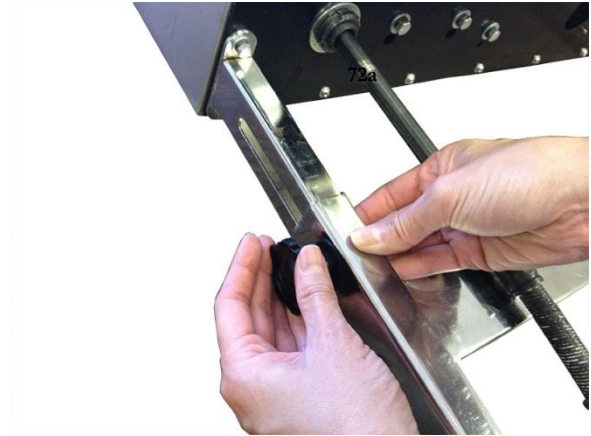
Figure 28. Tighten both sides with screw and knob. You can make adjustments to the height of your band sealer.
