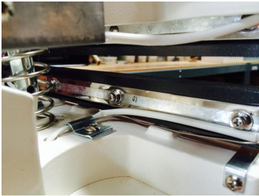
Figure 6. Loosen screws found on sealing jaw.
