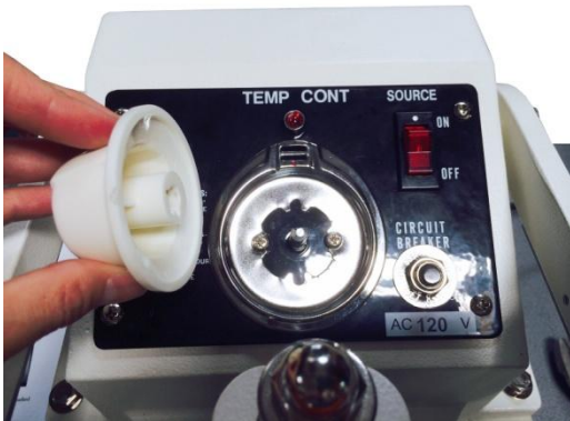
Figure 8. Remove thermostat cap.
