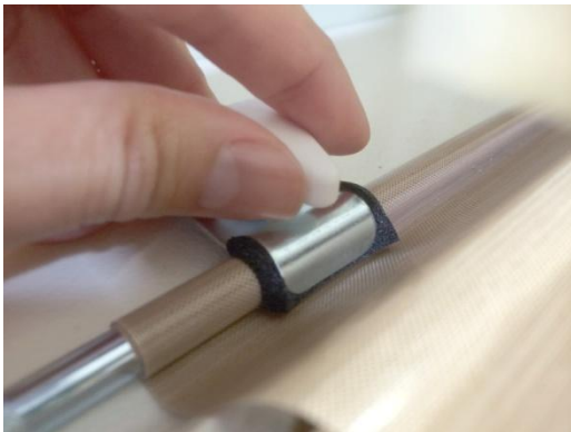
Figure 7. Loosen multi-star knob to remove the PTFE roller.
