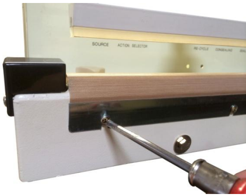
Figure 3. Loosen screws on PTFE plate.
