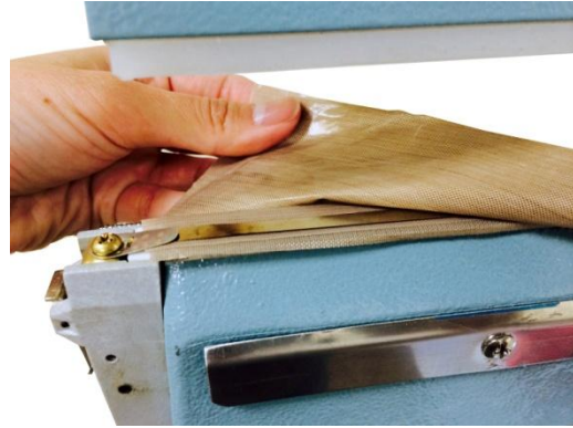
Figure 4. Pull PTFE cover to expose heating element.
