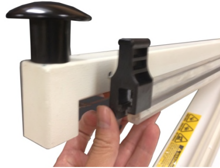
Figure 8. Slide the cutting bracket out.
