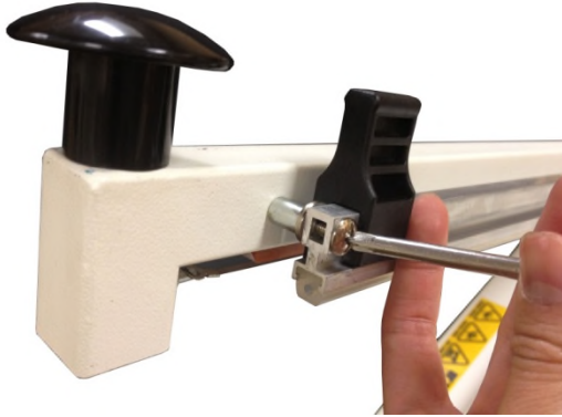
Figure 7. Unscrew the silicone bracket and remove screw, washer and spacers.
