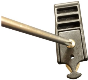
Figure 9. Remove cutter protector.
