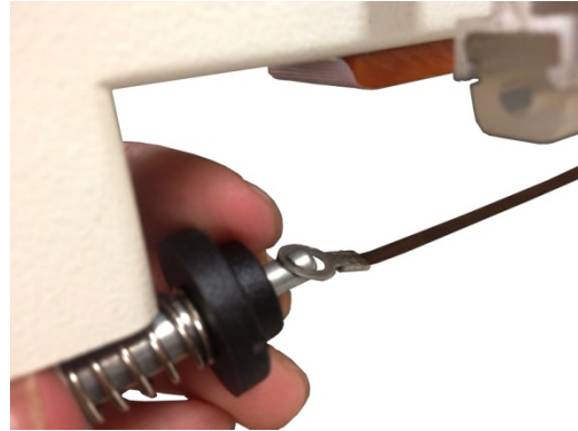
Figure 4. Remove heating element from spring hook assembly groove
