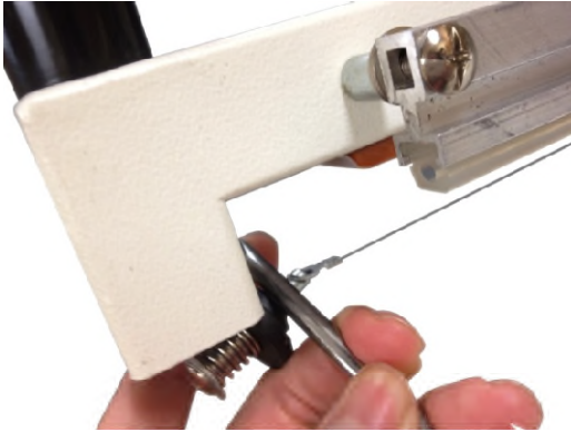
Figure 3. Using a screwdriver pull down spring hook assembly
