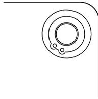
**2b.** Locate the hole on the drinking fountain pan surfaces. Align and sandwich with the two washers and tighten the nut to secure the bubbler.
