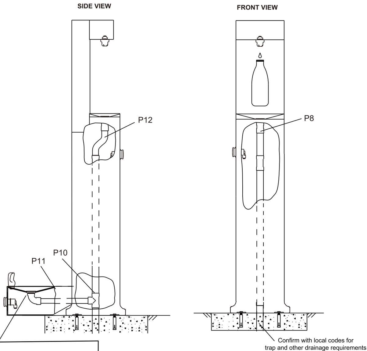
Reinstall access panel on the base of the pet station pan **BEFORE** connecting (P11) Drain Tube to (P10) T-Shape Drain Connector; using (4) M6 x 10 flat-head anti-theft screws precisely removed.
