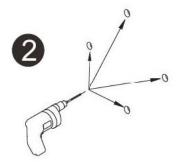
Drill the (4) holes 2" deep using 1/2" diameter concrete drill bit (Provided)
