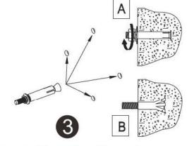
Insert the (4) expansion bolt into the holes Hammer down until the sleeve is level with concrete
