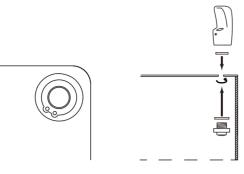
**2b.** Locate the hole on the drinking fountain pan surfaces. Align and sanwich with the two washers and tighten the nut to secure the bubbler.
