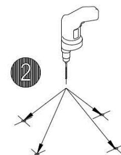
Drill the (4) holes 2" deep using 1/2" diameter
