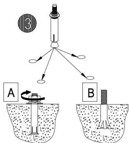
Insert the (4) expansion bolt into the holes
