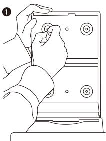
Position the dispenser against the desired spot on the wall where it will be mounted. Use a marker to mark the position of the outside four holes where the holes should be drilled. A spirit level should be used to make sure the dispenser hangs straight.
