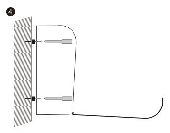
Insert the provided 1.4" inch screws through the dispenser into the provided black rubber distance holders which are placed between the wall and dispenser. Screw the dispenser into position.
