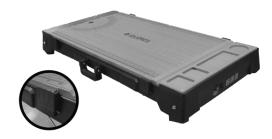
From Creeper mode, release the four latches on the sides of the workbench to flip platform panel to the non-slip surface side.
