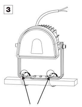
Use a flat head screw driver or socket wrench to tighten the clamp
