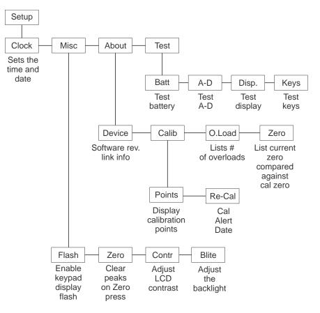
Figure 5.1 Operator setup menu
