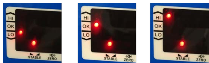
Figure 3 - C3236 limits annunciators: LO, OK, HI.
