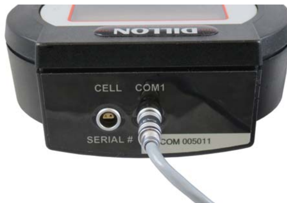
Figure 2.7 External Power Supply Connection (Communicator)
