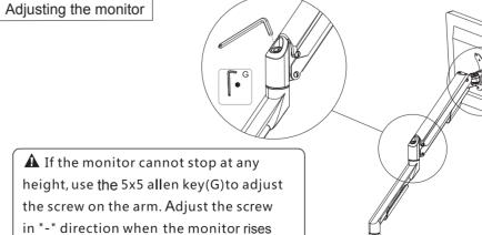
To adjust the swivel function use 5x5 allen key(G) on position 1. To adjust the tilt function use M6 box wrench(E) on position 2.
