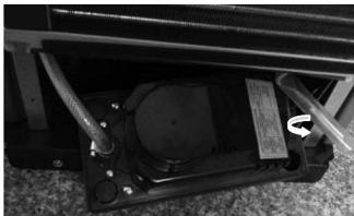
4. Remove screws (4pcs) to remove bottom cover then clean the water pump.
