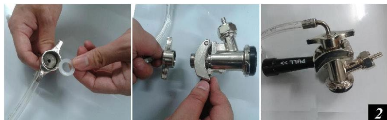
2. Thread beer line connector to keg coupler.
