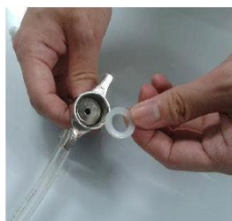
2. Thread beer line connector to keg coupler.
