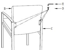
Step 2 Attach and hand tighten back cushion to the seat frame using screws. (Do not fully tighten screws)
