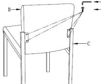
Step 2 Attach and hand tighten back cushion to the seat frame using screws. (Do not fully tighten screws)
