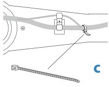
NOTE: Leave enough slack in cable to allow full range of motion.
