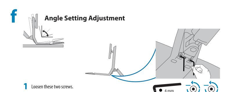
2 Loosen or tighten this bolt to adjust tilt to desired angle.
