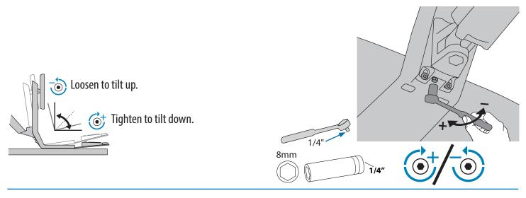
3 After desired tilt is achieved, retighten these two screws to secure.
