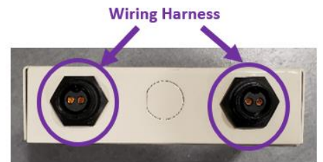
Figure 5 (Bottom of Control Box)
