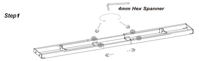
Loosen the 4 screws of the beam with the 4mm hex key. Then extend the beam to the proper position to fit the table top.
