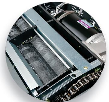
Chain-driven continuous duty motor for maximum power.
