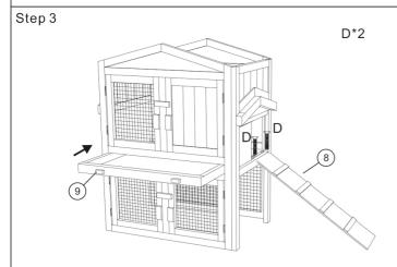
Secure 1x part® with 2x screw(D). Insert metal tray part®.
