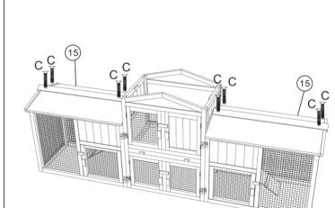
Secure 2x part (15) finished in step 1, using total 8x screw(C).
