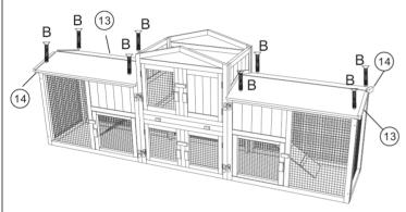
Attach 2x roof part (13) and 2x part (14) as shown, secure using 8x screw(B).
