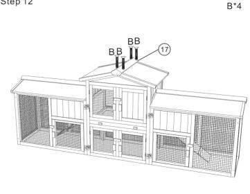
Attach roof cap part (17) finished in step 1, secure with 4x screw(B).
