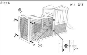
(1)Turn to back, attach 1x part(11), using 2x lock(E) to fix. Secure each lock(E) using 4x screw(D).
