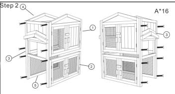
(1)Connect front panels part①,② to part③, secure with 4x screw(A) first. Then connect back panels part@and⑤, secure with 4x screw (A). (2) secure another part ③, using 8x screw(A).
