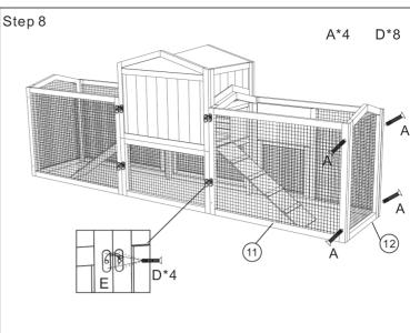
(1)Turn to back, attach another part 1, using 2x lock(E) to fix. Secure each lock(E) using 4x screw(D).
