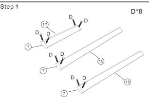
(1)Connect 2x part to part to, secure each side with 2x screw(D). (2)Connect 1x part 7 to part 15, secure with 2x screw (D). Repeat for another.
