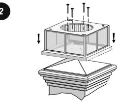
Place the lens housing on top of the post. Secure 4 screws through the holes in the solar cap adaptor plate (access through the circular hole in the lens housing).
