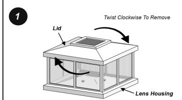
Remove the solar cap lid by holding the lens housing in place and then twist the lid in a clockwise direction. Be careful when twisting the lid to avoid damaging the tabs.
