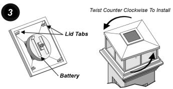
Be sure to pull the plastic tab from bottom of the lid to activate the battery (also check for correct orientation of the battery). Next, line up the lid tabs with the slots in the lens housing and twist counter clockwise to lock it in place.
