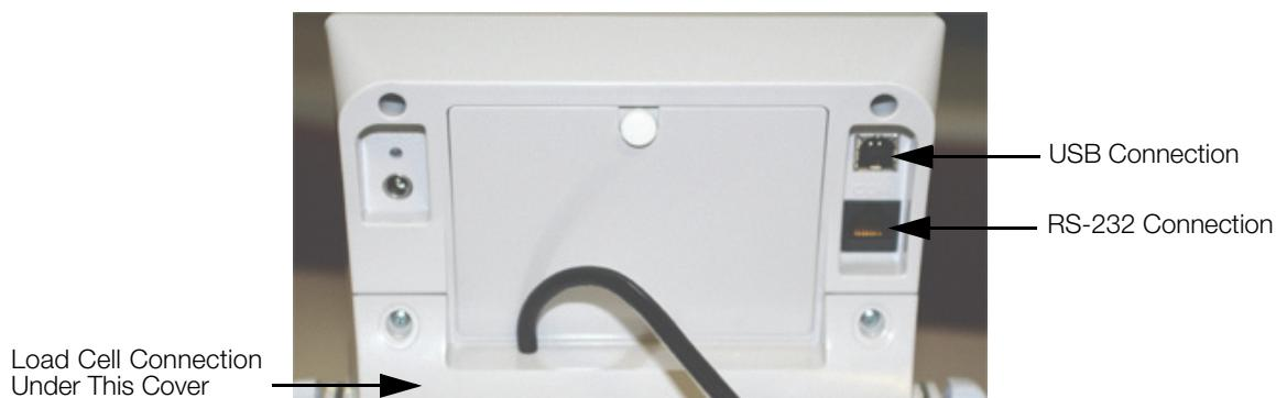
Figure 5-1. USB Connection Port and RS-232 Connection Port
