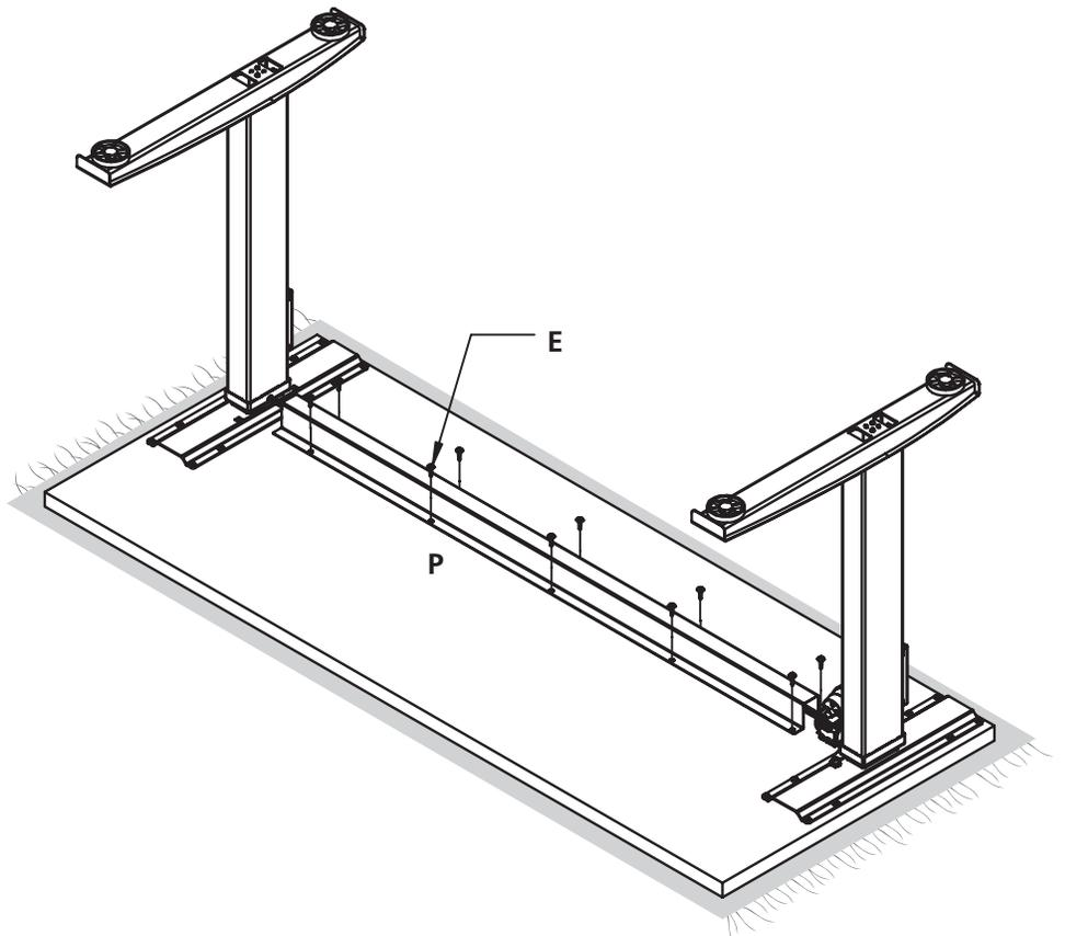
**Tip:** For proper alignment of pre-drilled holes, start screws but do not fully tighten until all are installed.
