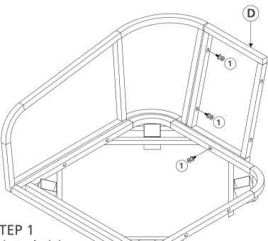
Connect part from STEP 1 & Back frame (D) with Bolt (1)
