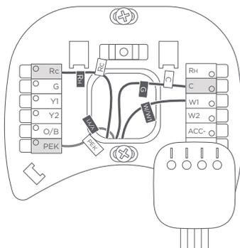
4. If you installed the Power Extender Kit, make sure you inserted the wires into the correct terminals.
