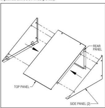
Step 3: Attach the sloping hood to the top of the locker with #10 - 24 x 3/8" slot less screws and #10 nuts (provided).
