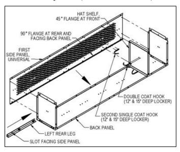
**Step 3:** Attach the second side panel and the right rear leg to the assembly of Step 2. On 12" and 15" deep lockers attach a third single coat hook. On 18" deep lockers substitute a single coat hook with a double bend for the third single coat hook and install the coat rod as shown on page 3. The locker chassis is now complete.
