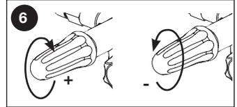
**NOTICE:** DO NOT overtighten the pressure control knob, if overtightened the knob COULD break and result in immediate loss of water pressure and costly repairs to the unit.
