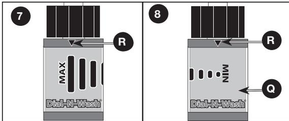
Adjust the pressure by rotating the Dial-N-Wash (Q) clockwise for higher pressure or counterclockwise for lower pressure, aligning the arrow with the desired pressure bar on the Dial-N-Wash.
